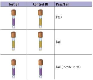
The steps using these tests are simple, and the results must be noted in the record book for documentation. A negative biologic indicator test gives a high level of assurance that the instruments were properly sterilized.
