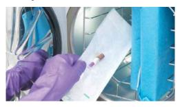
Assuming this strip is brown, after 10 minutes' cooling time has elapsed, both the test and the control vials are crushed and placed in the incubator for 24 hours. The operator can then view the color of the liquid in the test and the control vials – if the culture medium is still purple while the control test's culture medium is yellow, the test is negative, indicating sterilization occurred. If the color is yellow, the test is a fail (growth of spores has occurred during incubation).
