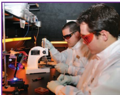
*This team is testing resin curing lights to determine their ability to cure a variety of resin-based composites.*
